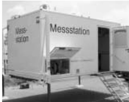
Agency for environmental Federal State of Bavaria Mobile laboratory with detachable shelter
